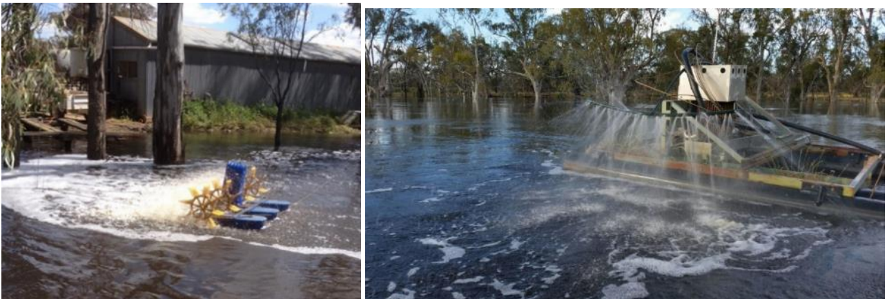
Figure 2: Left: Small aeration system deployed in the Edward River upstream of Moulamein to create a local fish refuge (Photo: Roger Knight 1/11/2016). Right: Improved aeration system installed by local landholder
